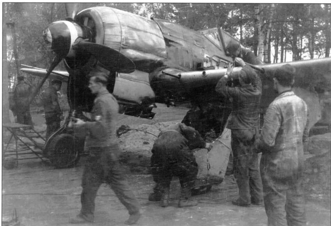
Armourers hastily attend to the reloading of one of the wing-mounted 20 mm MG 151/20 cannon fitted to a Sturmstaffel 1 Fw 190A-7 at Salzwedel in early April 1944. The fighter's spinner and cowling are streaked with engine fluid and gun muzzle deposits
