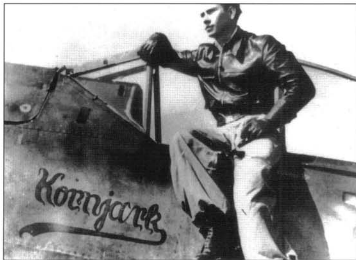
Another ex-eastern front veteran from JG 51, Feldwebel Konrad Bauer would become one of the most successful bomber-killers of the Defence of the Reich campaign. Note the small yellow ring (painted on the breech cover above the aircraft's name) which indicated that this machine was fitted with an uprated BMW 801D-2 engine
