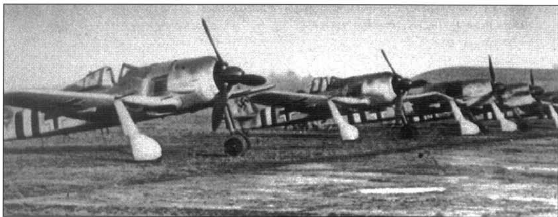
A line-up of fully armed and armoured A-6s shows off Sturmstaffel 1 's newly introduced and highly distinctive black-white-black aft fuselage bands
