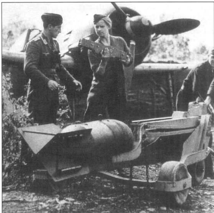
Armourers ready a 551-lb SC 250 bomb (which appears to be fitted with tailfin screamers) for attachment to a Sturmbock in preparation for a Jabo raid against the Normandy beachhead
