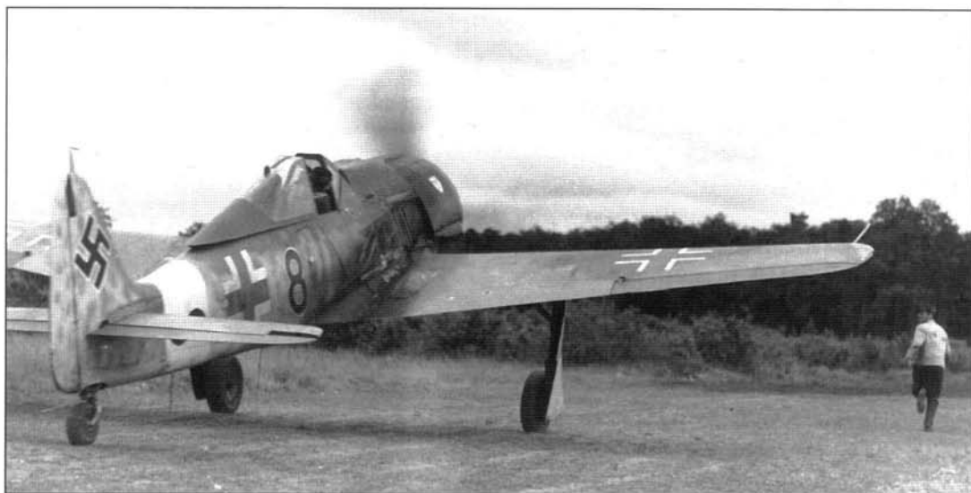
Blinkered or not, forward visibility from a Fw 190 when on the ground was non-existent. Willi Maximowitz peers cautiously out of the cockpit of his 'Black 8' as a mechanic runs just in front of the fighter, guiding the pilot towards one of the field's wooded dispersal areas
